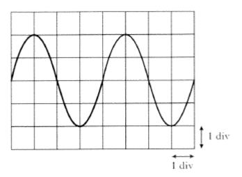
The timebase of the oscilloscope is set at 30 ms/div.
